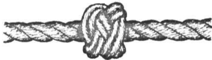
Fig. 23. – A shroud knot (fourth variation).
