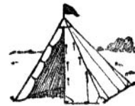
The wedge tent. It is shown suspended from an outside ridge rope.
